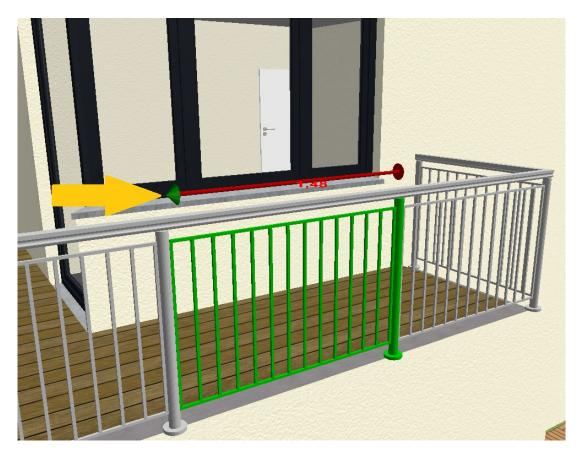
Double-click on the cone to open the dialog for entering the length numerically.
