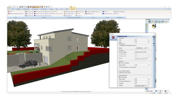
Retaining walls can have a fixed height, or a height that takes into account the terrain at the end of the segment and forces the segment to the specified value at that point. This also means that the height elsewhere is higher than specified in the dialog.
