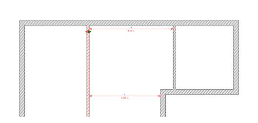
In this editing mode, you can change the direction by clicking on the respective part of the double arrow. A second click on the same part of the double arrow or on another part of the wall hides the moving dimensions and shows the usual dimension lines for the lengths again.
