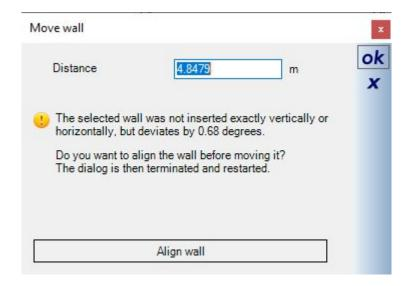
It is also important to mention that the displayed distance does not refer to the point at which the dimension line is displayed, but to the point at which the wall is intersected with another. An example to illustrate the position:
