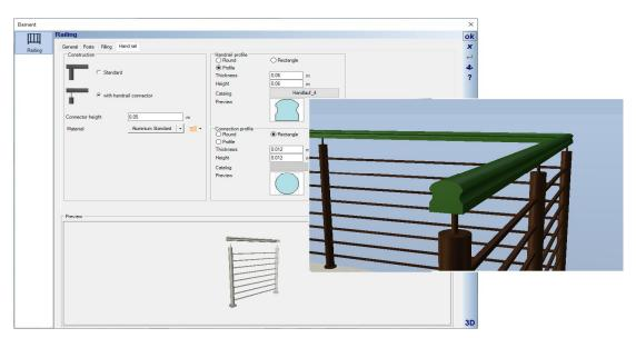
An example of a handrail profile with the associated representation in 3D.
