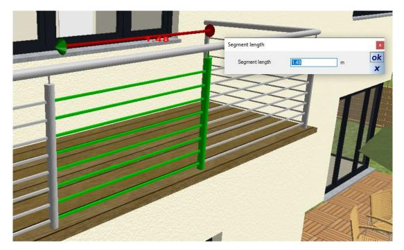
If a segment of a railing has been individually modified, the normal dividing options are disabled and the "Userdefined" checkbox shows this status.
