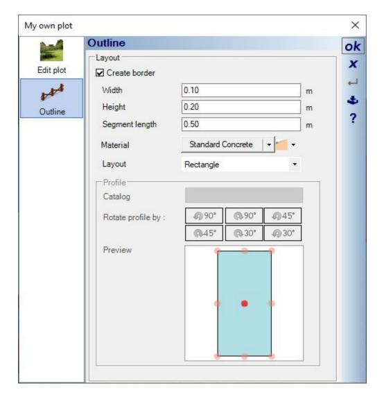
The border is all the way around, leaving no gaps for driveways or ways into the plot. It is really only intended to show the plot contour in 3D.
