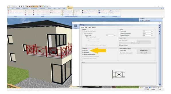
Here the railing with the same 3D object, but with an even segment length in the width of the 3D object.
